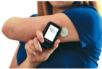
Fig. 3.1: Freestyle Libre sensor and reader in use[Noag].
